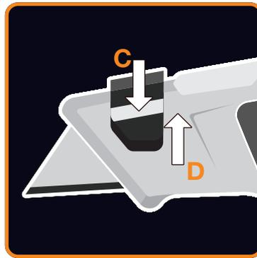
2. Push silver button on the black lock (C) and slide up until the blade is unlocked (D).
