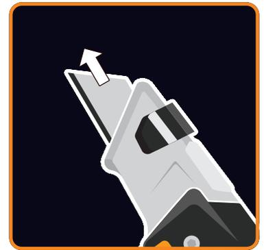
3. Pull the blade out of the front of the knife.
