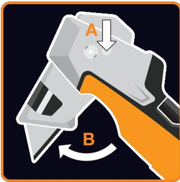
1. Press the button on the side of the knife (A) to flip knife to open position (B)
