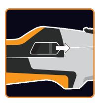
2. Slide the lock until the handle springs open.
