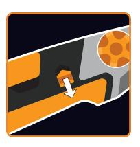
Push the lock down into the locked position.
