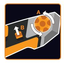
Turn wheel counter clockwise until it stops (A), then push the blade lock up (B).
