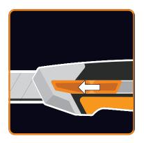
2. Push the blade slider out and make sure the blade is fully extended.
